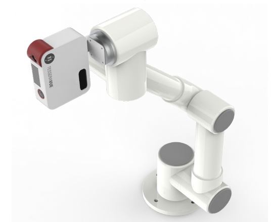
"TesseraVue": On-Device AI-Powered 3D Scanner Mounted on a Robotic Arm (Source: 4DiVISION)
